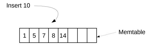
New insertions are kept in memory in a sorted buffer (memtable)
